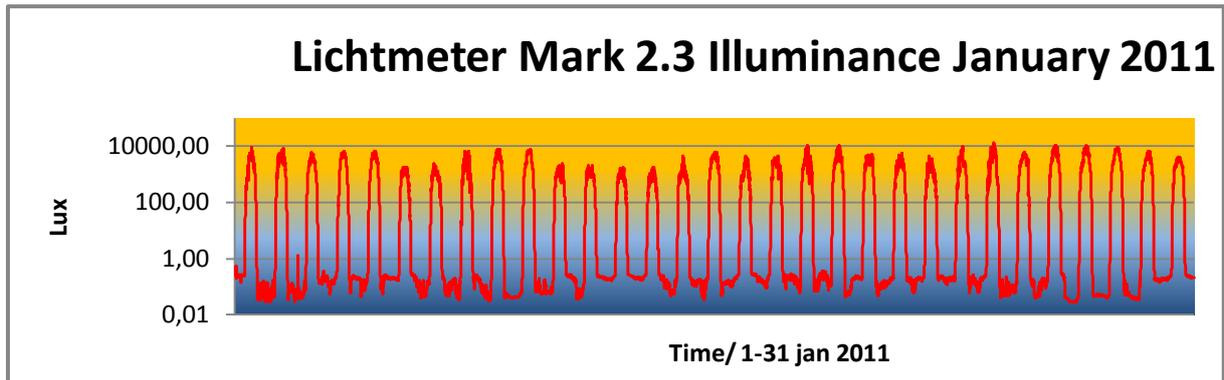
In the graphic above are the measurements of one month of the Lichtmeter Mark 3.2. The nights are visible by the low values and the days as the high values at the top. In January the sun does not come high and the highest values are around 10.000 lux; in the summer this can be 10 times higher. You can see also the nights are longer then the days.
