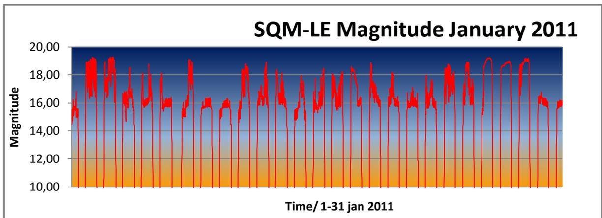
The graphic of the SQM-LE over the same month looks like this. The nights are the values around 18 and 19. The apparatus does not measure during the day. it switches off around magnitude 6, which is as the sun is a few degrees above the horizon.
